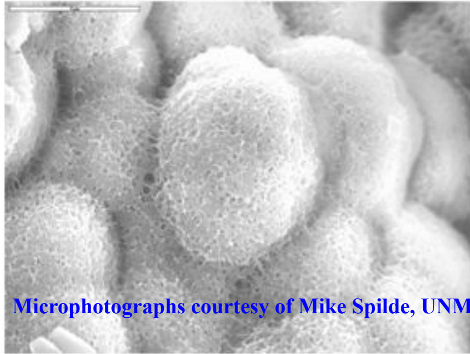
Figure 4. Surface of encrusted sample showing a globule at high magnification. Original magnification = 8000x; Scale bar = 5 \mu\text{m} .
